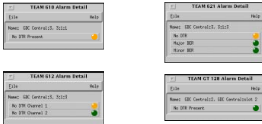
Figure 6-6 Alarm Detail Screens of the Remote Units
