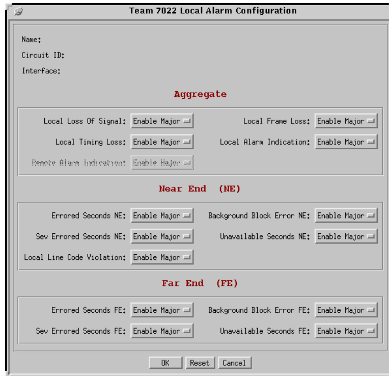
Figure 5-5 Local Alarm Configuration Screen (7022)
