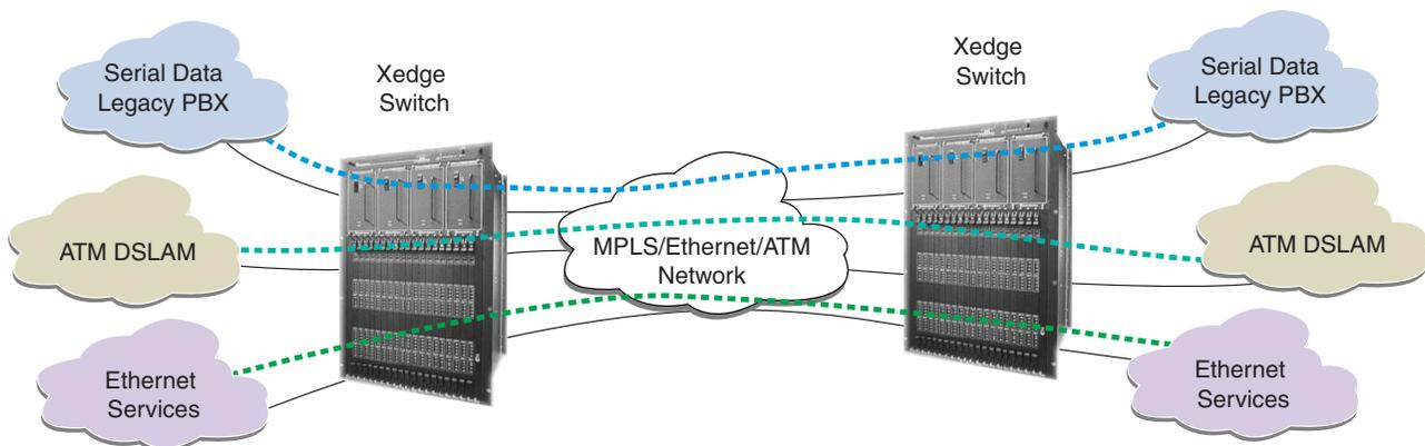
Figure 4: The Xedge MultiService Packet Exchange Platform
